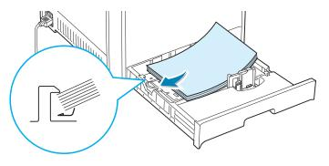
**3** Pinch the paper guide, as shown and move it towards the paper until it lightly touches the side of the stack. Do not push the guide to tightly against the edge of the paper as it may cause the paper to bend.
